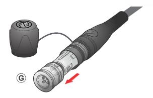
**9.** After the cleaning procedure unlock the NEUTRIK inspection tool (G).
