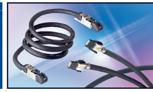
Belden® CatSnake™ Cat 6A tested cables deliver superior performance thanks to the 100% coverage of the pairs individually shielded with Beldfoil® aluminium/polyester foil and an overall braided shield.
