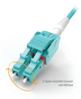
SENKO LC Duplex Switchable Connector is a unique design that allows the use of round style, 2.0mm or 3.0mm jacketed cable instead of the traditional zipcord duplex cable for a more compact design. The housing of the LC Duplex Switchable Connector can be taken apart in the without the use of any special tooling. This duplex LC allows the polarity to be switched at the time of cable assembly installation without having to re-terminate the connectors.
