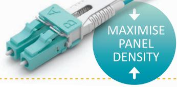
The SENKO LC-HD, is a totally unique design which can further increase panel density over currently available solutions and allow for the highest density possible. A gentle pull on the tab will disengage it from an extremely dense fiber optical panel. The pull tab is a perfect location to affix a connector label to help in the quick identification of the connector.
