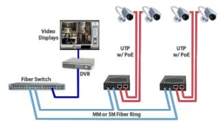
A third option is to have redundant f ber links for installations requiring fiber facility protection. There is an active f ber port and a protection fiber port that can support a f ber failure switchover of less than 50 milliseconds. The PoE+ media converter supplies power to the camera, and has power protection from an Uninterrupt ble Power Supply (UPS) battery back-up. In the event of a fiber cut and a loss of power, the camera continues to send data on the protection link.
